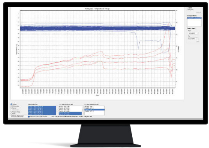
Figure 8 - Screenshot of Historical String (Cabinet) Temperature with Cell Voltages in a System in Thermal Walkaway
