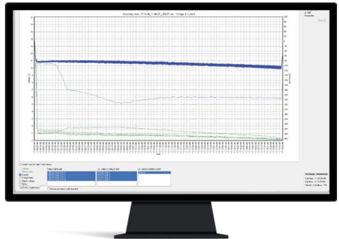
Figure 6 - Screenshot of Cell-Level Discharge Voltage Performance and String Current
