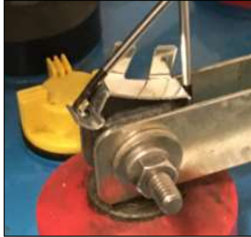
Installing a Post Clip using Screwdrivers
